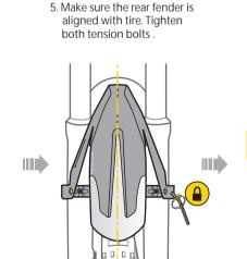
mm clearance between fender and tire as shown. Tighten ≥**35 mm** clearance
